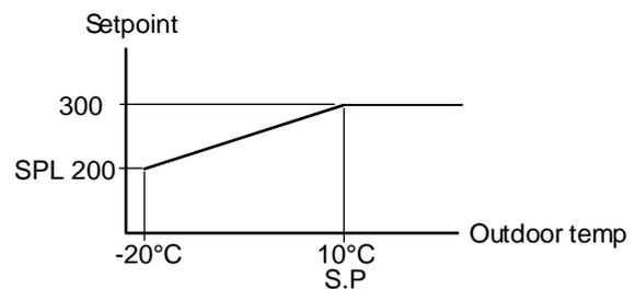
Example: With an ordinary setpoint of 300 Pa, a starting point S.P of +10°C and a SPL of 200 Pa at -20°C you get the following setpoint-to-outdoor temperature relation
