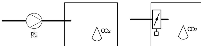
The output signal will increase when the CO<sub>2</sub>-value rises above the setpoint value.
